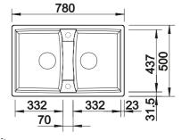
Pre-drilled holes for tapping or drilling Bowl depth 190/190 mm
