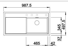
Pre-drilled holes for tapping or drilling Bowl depth 190 mm
