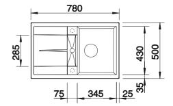
© Pre-drilled holes for tapping or drilling Bowl depth 190/25 mm
