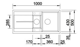
Pre-drilled holes for tapping or drilling Bowl depth 190/145 mm
