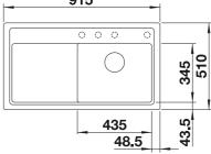
Pre-drilled holes for tapping or drilling Bowl depth 190 mm
