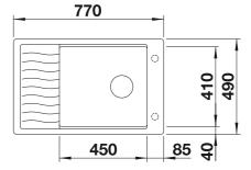
Pre-drilled holes for tapping or drilling Bowl depth 190 mm
