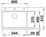
Pre-drilled holes for tapping or drilling Bowl depth 220 mm
