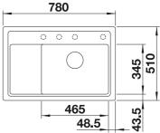
Pre-drilled holes for tapping or drilling Bowl depth 190 mm
