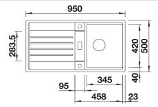
© Pre-drilled holes for tapping or drilling Bowl depth 190/50 mm
