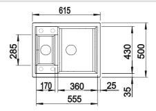
Pre-drilled holes for tapping or drilling Bowl depth 190/130 mm
