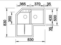
Pre-drilled holes for tapping or drilling Bowl depth 190/130 mm Cut-out by template.
