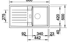
Pre-drilled holes for tapping or drilling Bowl depth 190/25 mm
