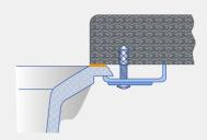
Special supporting elements are required for undermounting inset sinks.
