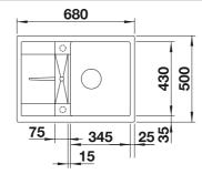
Pre-drilled holes for tapping or drilling Bowl depth 190/25 mm
