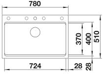
OPre-drilled holes for tapping or drilling Bowl depth 220 mm
