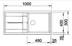
© Pre-drilled holes for tapping or drilling Bowl depth 190 mm
