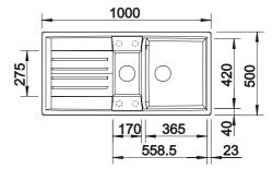
Pre-drilled holes for tapping or drilling Bowl depth 190/145 mm
