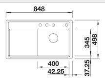
© Pre-drilled holes for tapping or drilling Bowl depth 190 mm
