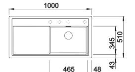
○ Pre-drilled holes for tapping or drilling Bowl depth 190 mm
