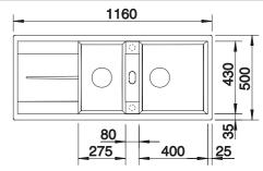
© Pre-drilled holes for tapping or drilling Bowl depth 190/190 mm
