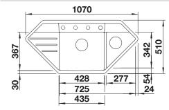
Pre-drilled holes for tapping or drilling Bowl depth 190/130 mm Cut-out by template.
