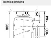
3 1/2" sink outlet required. Product weight: 10,6 kg. Non-detachable 90 cm power cord. Reset-button on bottom of the FWD (note accessibility)
