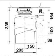
3 1/2" sink outlet required. Product weight: 11 kg. Non-detachable 90 cm power cord. Reset-button on bottom of the FWD (note accessibility)
